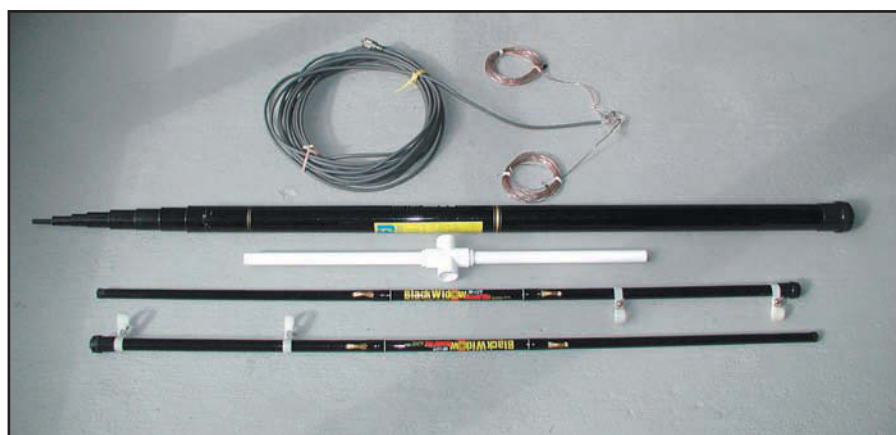
Figure 7—The completed antenna broken down for storage or travel.
